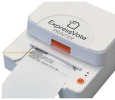
[This device](#) works with the e-pollbook to generate an “activation card”—a card with a bar code that identifies the correct ballot for the voter. The poll worker inserts a blank activation card into the printer, which is hard-wired to the e-pollbook. The printer prints the bar code identifying the correct ballot information on the card. The voter takes this card to the voting machine.
